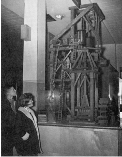
FIGURE A.21 Model of water pumping mill designed by Leonardo da Vinci. (Courtesy of Museum of Science, Boston, MA.)
