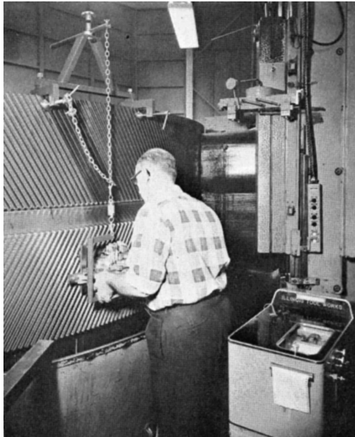
FIGURE 7.55 Portable profile-checking head mounted on the rim of a large gear. (From General Electric Co., Lynn, MA, USA.)
